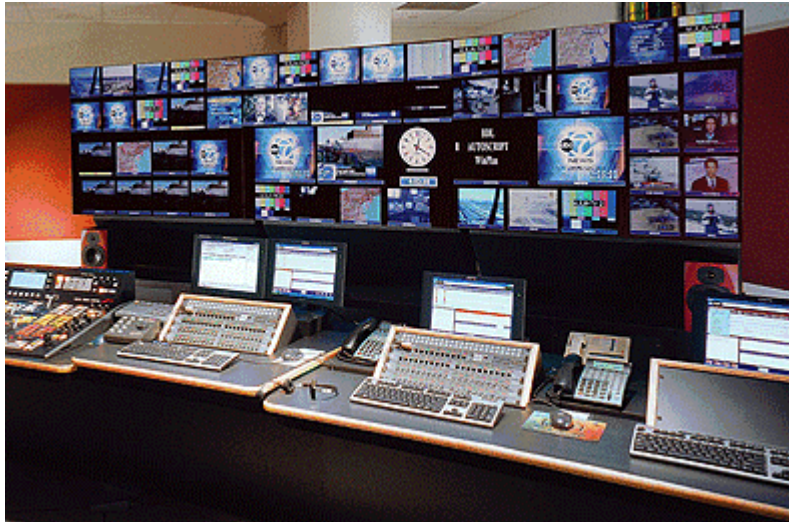
Picture 1 - Multiple monitors are tied together on a monitor wall to create a very large viewing experience.
